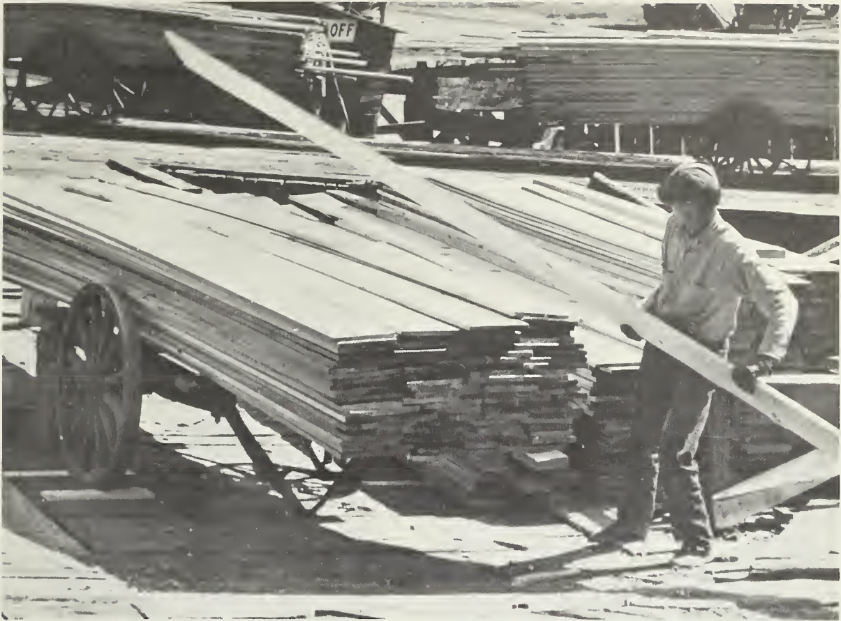
Figure 27. --A simple wagon for hauling green lumber to the yard.
